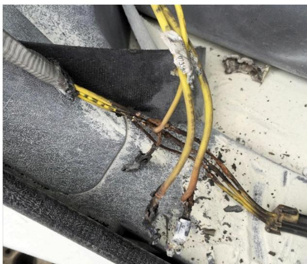
**Figure 6:** Overheated terminals at a relay started this minor fire.
