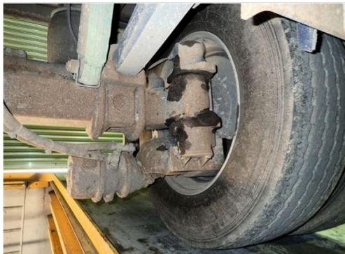
**Figure 21:** Low slung disc brake actuator.
