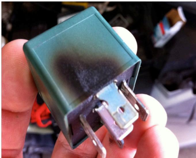
**Figure 7:** Overheated terminals at a ¼” blade nominal 30A relay
