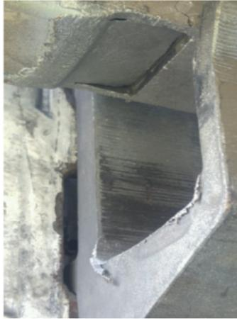
**Figure 26:** Rubbing between the mezzanine support bracket and beam leading to generation of hot metal fragments.
