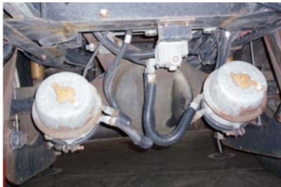
**Figure 22:** Low slung air hoses – vulnerable to damage.
