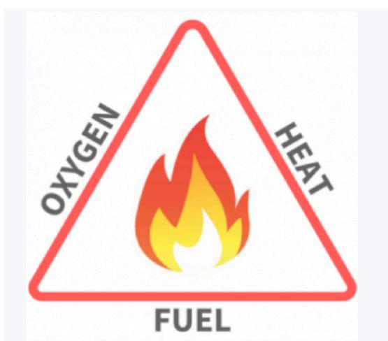
**Figure 3:** Fire Triangle – remove any element, stops a fire
