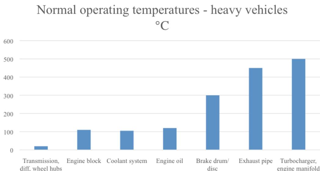
**Figure 4:** Normal operating temperatures for heavy vehicles
