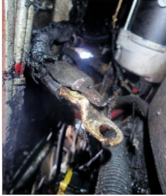
**Figure 9** The main return cable was left off the starter motor.
