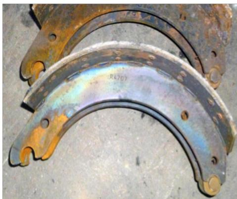
**Figure 20:** Trailer drum brake shoes showing destruction of linings due to dragging brakes
