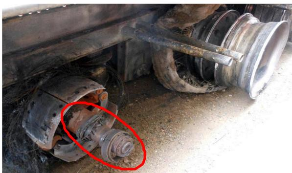
**Figure 24:** Failure of wheel bearings on the front axle resulting in a trailer fire
