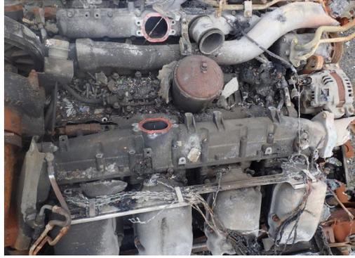
**Figure 17:** An engine failure resulted in the engine cover breaking. In this case an engine failure caused an oil leak into the turbo-charger.
