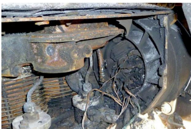
**Figure 8:** The accumulation of grain dust around the alternator on this blower motor resulted in a leakage of current via carbon-rich dust that developed over time into short-circuit and caused a fire.
