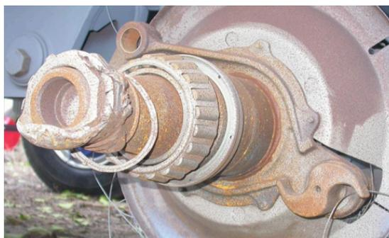
**Figure 23:** Failed outer wheel bearing
